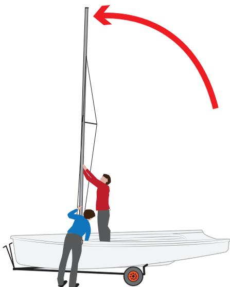
You can now lift the mast up over the gunwhale of the Venture, keeping it upright of course, and rest it down in the bottom of the boat, just aft of the mast step.
