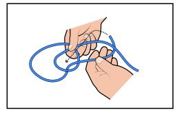
Thread the tail back through the loop, and tighten
