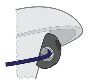
This retro kit allows you to remove the mainsheet ratchet and add a swivel base easily, which can still be removed to stack boats together.
