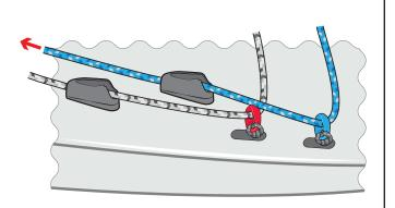
Pass the end forward to the front (double) block on the starboard organiser by the mast step and rig the downhaul purchase as shown.
