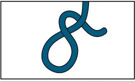
Lead the tail of the rope back through the loop, and tighten
