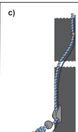
To keep things neat while stepping the mast you can add the main halyard and tail to the lower cleat.
