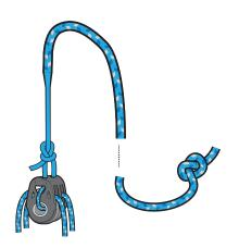
Attach the tapered end of the downhaul tail onto the double block with a bowline.
