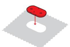
Place the thicker base plate on the deck with it's undergrooves pointing inboard. It is positioned in the gap in the non-skid. There is a wooden block underneath.
