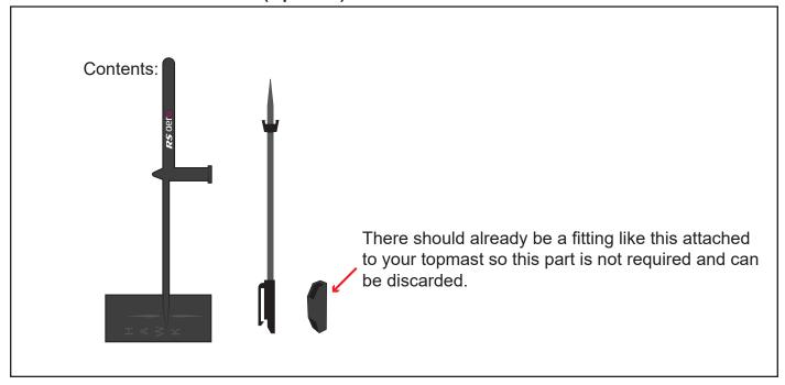
Clip the 2 parts of the wind indicator together
