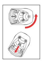
Rotate the fitting so the cleat in aligned fore and aft and then push/strike it forward until the fitting clicks into place.
