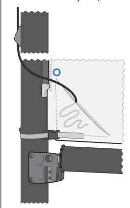
Feed the downhaul through the eye on the tack of the sail from starboard to port and tie an overhand knot.
