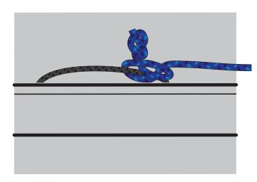
**b)** Tie two figure of eight knots 1/3 and 2/3 of the way down the blue rope.
