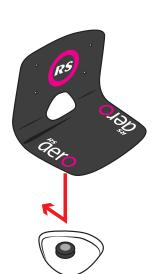
• Clip the compass bracket onto the button.
