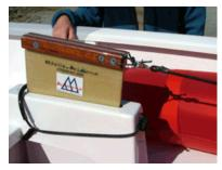
wind. It requires two-hand operation. This system only requires one hand for precise height adjustment with minimum effort. The Optisailors hull has a second "bungee" line that attaches to the mast thwart from the top of the daggerboard. This exclusive **Optisailors** design helps eliminate the friction caused by the standard system and ensures that the board will be tied in (legal) during racing. The board is cock aft while up, which is preferred for low helm and speed.
