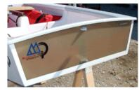
stiffen the boat. Extra care is taken to assure the maximum weight can be placed in the midship frame lightening the ends. The center of gravity is moved aft through a special vacuum bagging process. The **Optisailors** hull is perfectly faired. A clear transom option is also available for customers wanting to further distinguish their boat.
