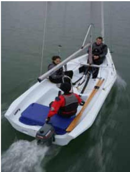
**The engine should be secured to the eye bolt with a piece of rope. This rope should be as long as possible without fouling the prop when the engine is running. A short lanyard can be a hazard if the engine comes loose from the bracket as the engine can turn over and the prop will be in the air.**
