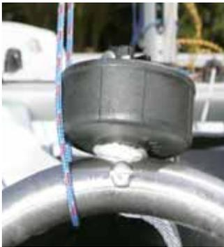
1. Ensure furling drum line is fully wound completely onto furling drum before you attach the jib.
