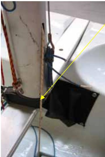
2. Ensure the end of the gennaker halyard taken from the base of the mast is free of knots and tangles.
