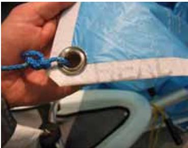
12. Untie the gennaker halyard from the lower shroud and secure to the Head of the gennaker using a bowline.
