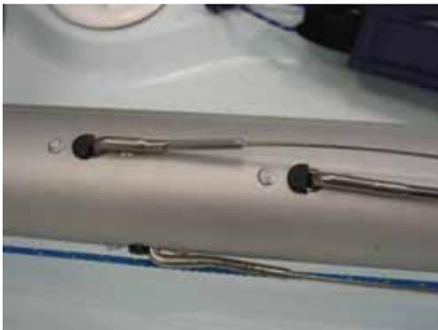
4. If applicable, fit trapeze wires and plugs in the top terminal positions on the mast. (Note: Trapeze kit is an option)
