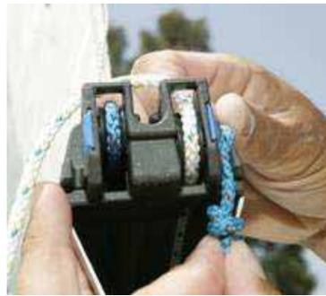
4. Outhaul tension is controlled using the blue rope, cleat and fairlead at the forward end of the boom.
