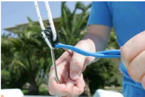
14. Attach the trapeze rings to hull mounted shock cords by feeding the elastic loop through the ring at the bottom of the pulley. (Note: Trapeze kit is an option)
