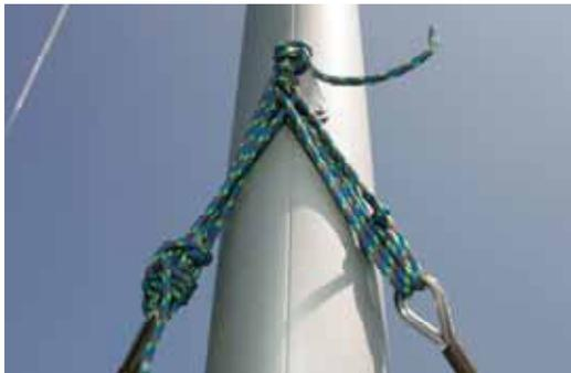
13. Loosely tie the other end of the lower shrouds to front of mast. **(Note: The lower shroud tension is adjusted after the jib halyard has been tensioned.)**
