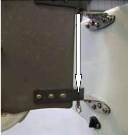
The pin goes through from the top of the rudder stock and through both sets of Gudgeons. This must be secured with the split ring below the bottom gudgeon.
