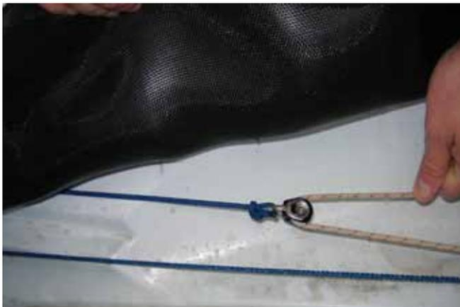
6. Feed the pole "out" rope and block back down the Shute towards the back of the boat.
