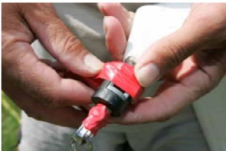
3. Attach the head of the jib to the jib halyard furling swivel and tape up prior to hoisting.
