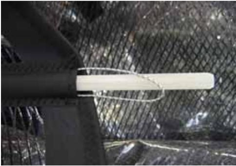
a. To release the tension from a batten, slide the batten prodder (supplied) carefully between the two halves of the velcro locking mechanism and pull the retrieval line slowly.
