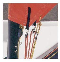
exiting from the bottom of the boom near the gooseneck. Zip up the mainsail sleeve.
