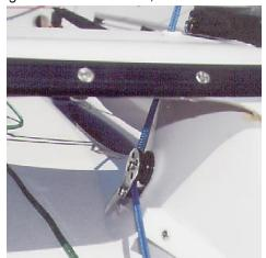
the line inside the spin pole and the pole extension line. See photo below. From there, it continues forward and passes through the larger of the two
