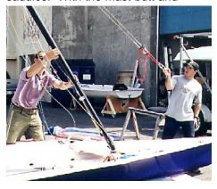
shrouds connected, make sure the trapeze wires are in an unobstructed position where they can help pull the mast to its upright position. Use both trapeze wires to pull the mast upright as the person holding the tip walks it up beside the boat until out of reach.
