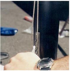
wire loop on to the teeth on the rack mounted on the side of the mast. Typically you will be on the first or second hook. Loop the clew tie-down over the end of the boom and attach the outhaul hook. (See earlier picture on p.2) Set the vang ram on the boom, and tuck all the halyard ends neatly inside the mainsail pocket.
