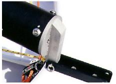
stern. With one person holding the tip of the mast so that it is about a foot off the transom, (or resting it on a horse), attach the butt to the hole in the step.
