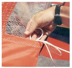
At this point you can attach the downhaul (Cunningham) hooks to the bottom of each side of the mainsail making sure that there are no twists in the purchase to allow for unencumbered adjustment. Also attach the vang adjustment hook to a bowline tied in the end of the vang shoe control line
