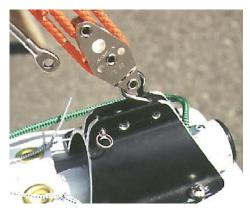
chase system supplied with the boat to the front hole of the bow plate.
