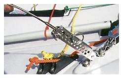
that if one end gets worn from use, it can be rotated instead of replaced. Remove the bottom pin from each chain plate, leaving the shrouds in place, and attach the end of the chain plate to the saddles mounted on the boat. The spinnaker sheet ratchet blocks are attached to the same saddles. With the mast butt and
