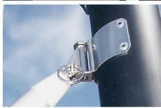
neck slightly below the beginning of the mainsail track. The lower end of the strut is attached to a "shoe" which should rest on the top of the boom and
