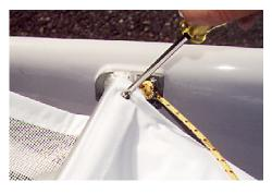
The first step is to lead the spinnaker halyard from where it exits the bottom of the mast straight down through an eye in the partner where it then passes forward through the cheek block mounted directly below on the side of the mast support. See below. It then goes towards the bow, UNDER both
