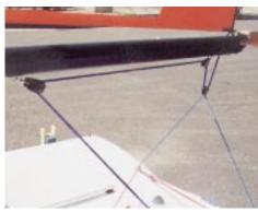
knot tied to the small saddle (deck strap). The final part passes through the block on the traveler and is tied off on the clew board (shown here being held by hand in the photo). The rules allow a shackle or quick release device for attachment to the clew.
