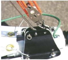
forestay to the CENTRE hole in the bowplate. Remove boom vang. If set correctly, the rig tension should measure around 28 on a Loos gauge.
