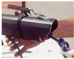
the end of the boom, just behind the hanging block. Pass the line up through the hole, out the back and put a figure eight in the end. (Note in the picture the arrangement of the clew loop and the outhaul hook block). The sheet then goes (photo above right) through the bridle traveler block, back up to the rear mainsheet hangar block on the boom, forward THROUGH THE
