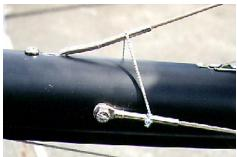
connect the forestay to the mast by first passing it underneath the small shock cord attached to the shrouds near the jib halyard sheave. The shock cord prevents the spinnaker halyard from getting caught in this area. The forestay should be taken off the mast while travelling as it is sticks out beyond the mast step and has been known to fall out of the key slot. Undo the spinnaker halyard and make sure there are stopper knots in both ends! Now!
