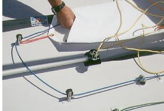
cockpit, passing under everything including the partner, through a small eye leading to the spinnaker halyard cleat and through the cleat. It goes straight back through a stand-up block and then over to the port side of the boat where it passes forward through another stand-up block. After passing through this block, this same halyard turns into the retrieval line for the spinnaker! Feed the retrieval line
