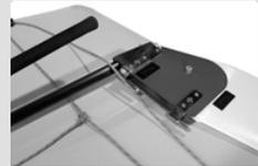
Allow plenty of slack in the traveler line before sliding the entire tiller and extension under only the traveler line that is connected between the two fairleads. Slide the rudder head back and insert the pintles of the rudderhead into place. Tighten the traveler line so that it is taut but still allows the traveler block to move freely across the traveler, clearing the tiller.
