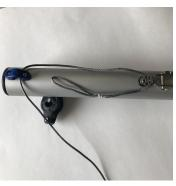
**4** - Pass the dyneema loop through the clew shackle w/ block and lead back to fairlead.
