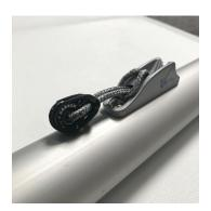
**2** - Attach block with closed loop to boom cleat by luggage tagging around cleat base.
