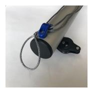
(7 - Derigging Note) - To release, simply pop the loop off the end of the boom and reverse the process above.
