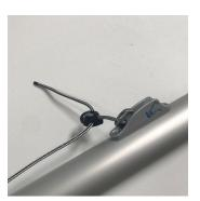
**8** - Take the free end of the control line and pass through the block that is attached to the boom cleat.
