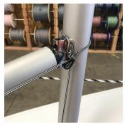
**10** - Finish rigging the outhaul by running the control line to the dangle block at the gooseneck, and then down to your deck blocks and cleat.
