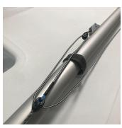
**9** - Pass the control line aft, through the block with the dual splices, and then forward towards the bow of your boat. Be sure to check for twists to minimize friction when tightening or releasing the control.
