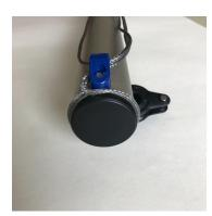
**6** - Push the loop over the end of the boom, locking the loop in place.
