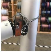
**1** - Attach the dangle block to the mast at gooseneck by slipping the block through the spliced loop.
