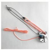
**9** - Finish rigging the cascade with the control line, passing the line back and forth between the vang base and the double block, and then down through the lower turning sheave and cam cleat.
