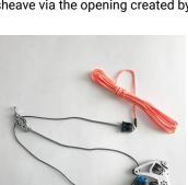
**8** - Pull the line away from the block - the control line cascade should be \*above\* the dyneema primary line.
