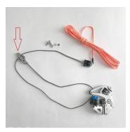
**7** - Slide the free end of the dyneema primary onto the sheave via the opening created by the removed key.
