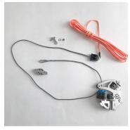
**3** - Pass the dyneema primary line (with loop) through the single turning block on the vang base (bottom to top) and pull away from the vang base.
